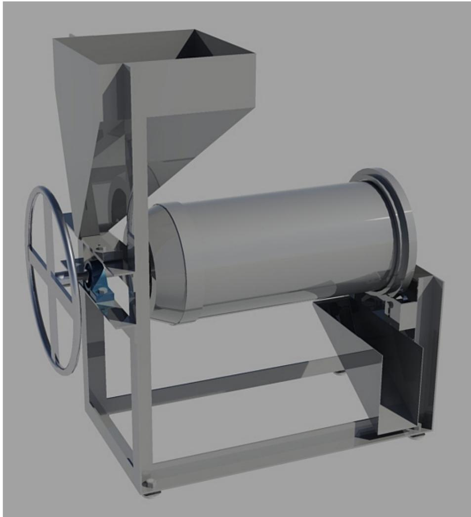
Prototype of redesigned rice length grader with manual option.
