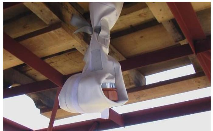
*Underneath the GrainSafe showing the tied downspout. Loosen the tie to start discharge of grains.*
