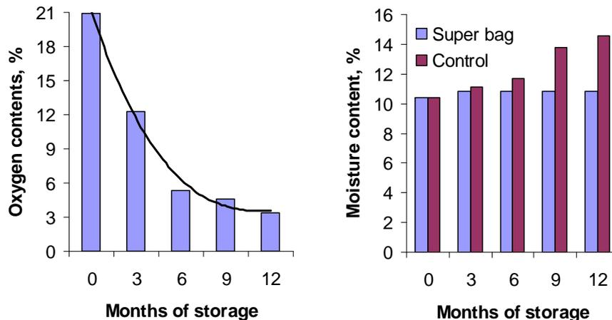
Figure 1: Oxygen contents in the Super bags (left) and moisture content in Super bags and the Control after 3, 6, 9 and 12 months of storage.
