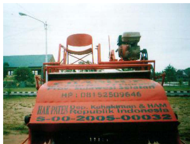
Fig. 3. The DP 7000 stripper harvester (Note the prominent display of the patent number and the seat for the operator).
