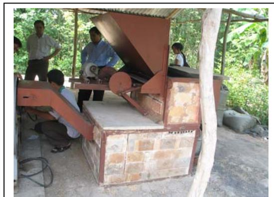
A prototype of the Automatic Rice Husk Furnace that is attached to the 4ton flat bed dryer.
