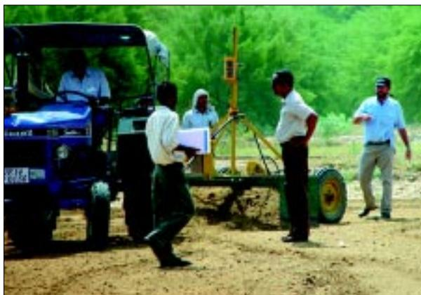
Fig.6. Laser leveler attached to a 4-wheel tractor.
