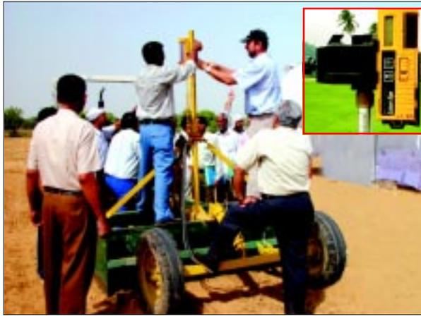
Fig. 11. Laser receiver being adjusted on the mast. Inset picture shows a close-up of a laser receiver.
