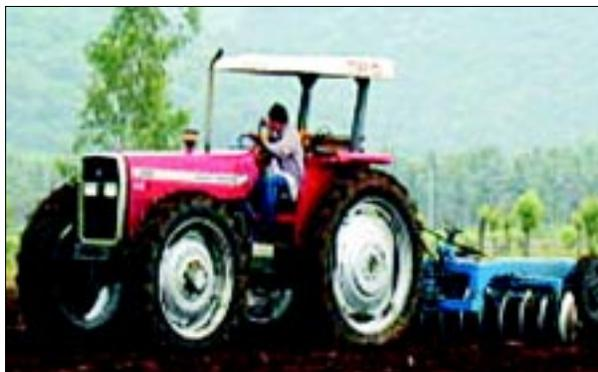
Fig. 9. Disc harrows being used to loosen hard layers exposed due to shifting of soil.
