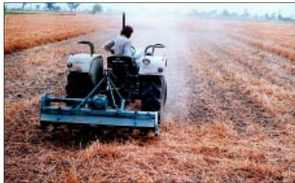
Fig.15. A rotovator is being used to cut up the surface residues.
