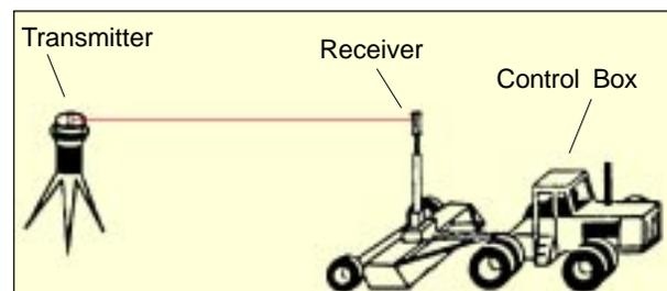
Fig.7. Diagram showing major components of a laser leveling system.
