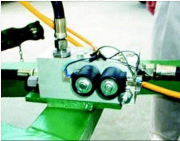
Fig.14. Hydraulic control system.
