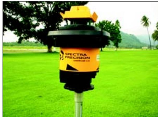
Fig.10. Laser transmitter
