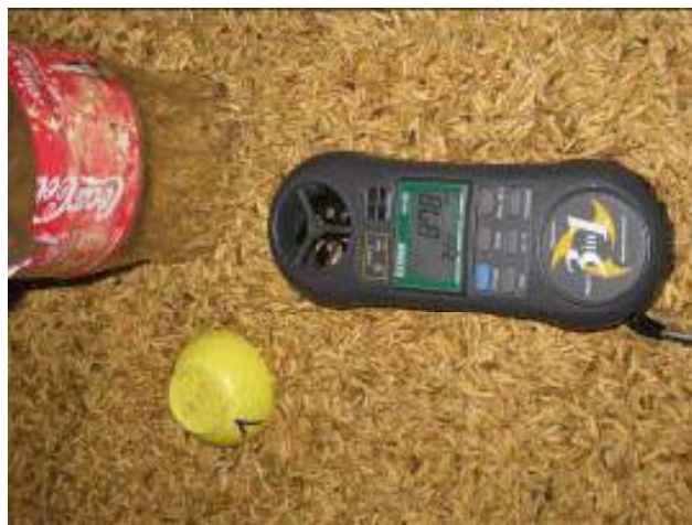
Measurements of temperature, velocity and RH of drying air using an anemometer
