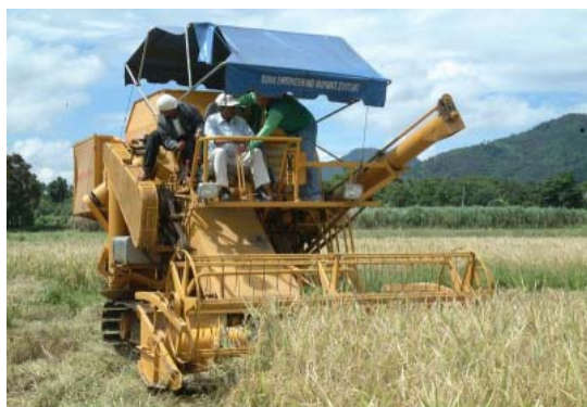
Thai combine: cutting width 2-3m, capacity 0.6-1ha/h, weight 4-8t
