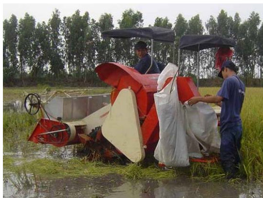
Mini combine: cutting width 1.2m, capacity 0.12 ha/h, weight 0.5t.
