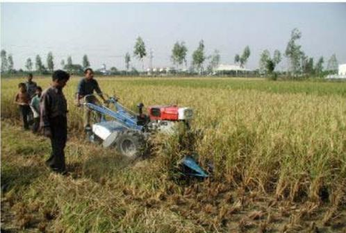
Cutting can also be done mechanically by a reaper, although the use of reapers is not wide-spread in Asia. In some countries, reapers are used that are mounted on the front of a tractor. Most reapers lay the crop in a windrow, which allows for easy pick up of the harvested crop. A reaper with a cutting-width of 1.5m can operate at a rate of 2-4 ha per day. For proper operation of reapers, fields need to be leveled and drained. It is difficult to reap crop that is lodged, lying on the ground.
