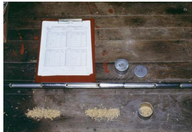
Figure 1: Probe, sample containers, and protocols
