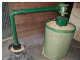
View on seed dryer during performance test
