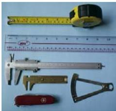
Standard tools for machine component and grain sizes are calipers in various forms.
