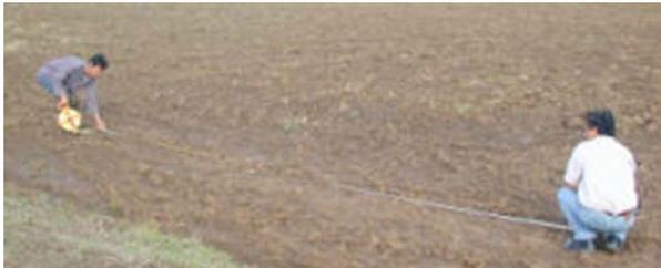
Made of steel, fiberglass or plastic tape measures vary from 1 to 200 meters in length. As most discrepancies occur at change stations, the longer the tape measure used the more accurate will be the distance measured.
