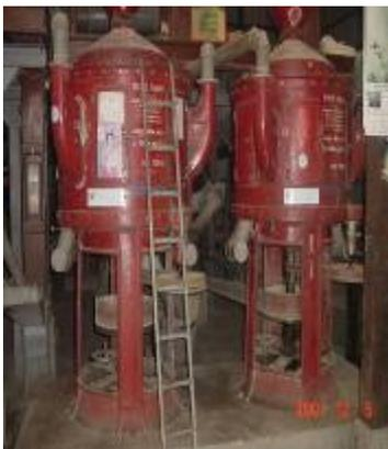
The process used to whiten brown rice can be classified as either abrasive or friction.
