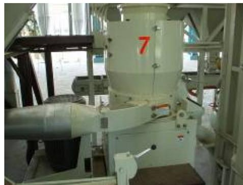
**Abrasive:** In this process the grain is whitened by the abrasive action of the rice kernel passing between a moving abrasive surface and stationary screen. The hard rough surface is usually stone or a carborundum type material. The abrasive process applies less pressure on the grain and is better suited for long grain varieties. Abrasive polishers can be either vertical or horizontal in design. The vertical cone whitener is very common in many Asian countries.
