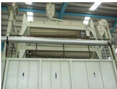
To attain a higher degree of precision for grading and separation, a length or indent grader is also used. This machine is made up of 1-3 rotating indented cylinders. The broken and smaller rice pieces fall into the indents on the rotating roller surface and are removed leaving the whole rice kernels or head rice.
