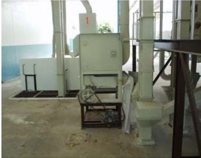
*Single drum with aspirator and oscillation sieve.* The single drum aspirator utilizes a single drum to separate large, light and heavy impurities. Lighter impurities are separated by suction aspiration and the oscillation sieves separate heavier impurities such as sand.
