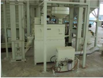
Mixing a fine mist of water with the dust retained on the whitened rice improves the luster of the rice (polishes) without significantly reducing the milling yield. A friction type-whitening machine, which delivers a fine mist of water during the final whitening process, is used for “final” polishing before sale.
