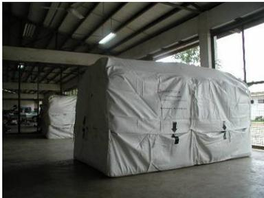
Sealed or hermetic storage systems are a very effective means of controlling grain moisture content and insect activity in tropical regions. These systems vary in size from 1-300 tons. By placing an airtight barrier between the grain and the outside atmosphere the moisture content of the stored grain will remain the same as when the storage was sealed. Smaller 50kg hermetic bags which fit inside the traditional bags are also available
