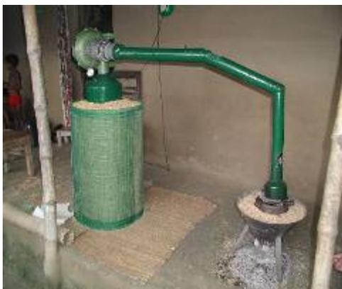
Rice is also dried in mechanical batch dryers. The most common smaller dryers have a capacity of 1-3 tons per day with drying times of 6-12 hours. For drying seed in tropical areas, an air temperature of 40°C-42°C is normally used with a heater capable of raising the air temperature 10°C-15°C. An air velocity 0.15-0.25m/s is required and typical power requirements are 1.5-2.5 kW /ton of paddy. The efficiency of these dryers is also improved by stirring the grain.
