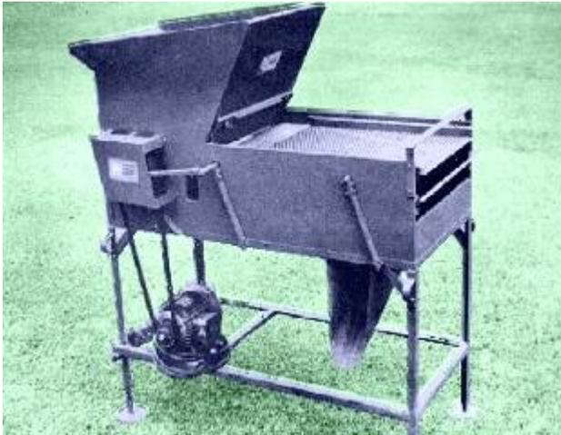
Mechanical winnowers that incorporate a fan and several superimposed reciprocating sieves or screens are now used in many countries. These can be manually powered or motorized and have capacities from 100kg to 2-3 tons per hour. Where combine harvesters are used, there is a trend towards using large capacity centralized seed cleaners. These are normally equipped with a series of vibrating sieves and are capable of 10-30 tons per hour.
