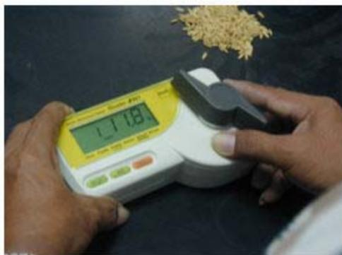
The secondary method uses electronic moisture testers.
