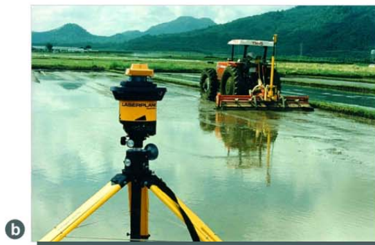
Figure 3. (a) Schematic diagram of laser operation. The control box activates the tractor hydraulic system to raise, lower or maintain the height of the tillage implement base on the horizontal laser beam. (b) Actual laser field operation. The precision (laser) leveling system for puddled soil was developed by Spectra Precision and IRRI.
