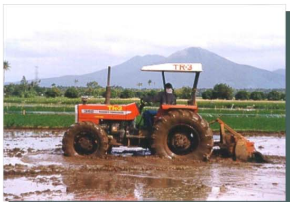
Figure 2. Shallow (a) dry and (b) wet tillage reduces power requirement and improves trafficability.
