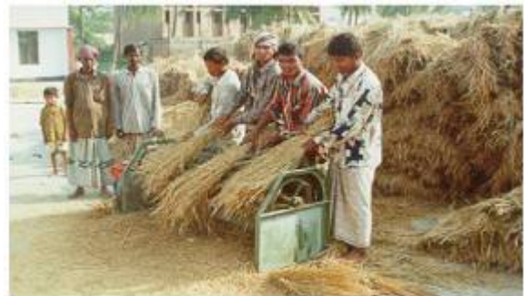
Figure 10: Threshing with a Pedal Thresher
