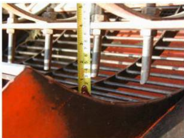
Figure 14: Checking the concave clearance
