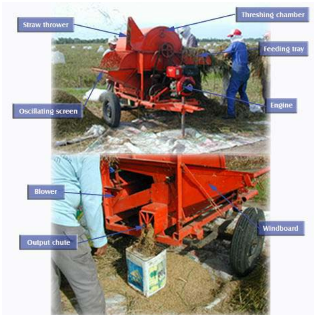
Figure 12: Components of an axial-flow, feed-in thresher with a cleaner
