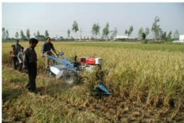
Figure 9: Reaper mounted on Chinese power tiller
