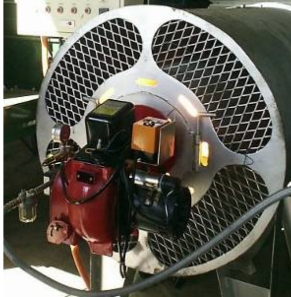
Figure 26: Kerosene burner attached at air heater of a re-circulating batch dryer
