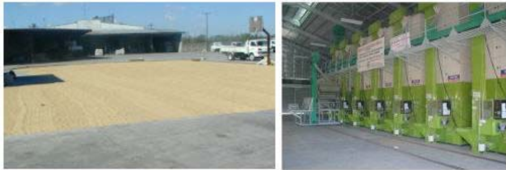
Figure 1: Sun drying pavement and re-circulating batch dryers, both installed at a rice mill
