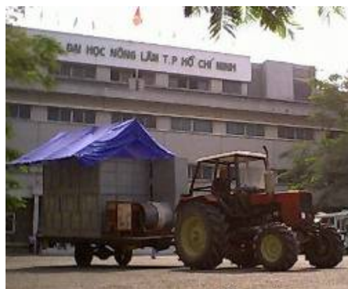
Figure 16: Principle (left) and example of a mobile reversible-flow batch dryer (right)
