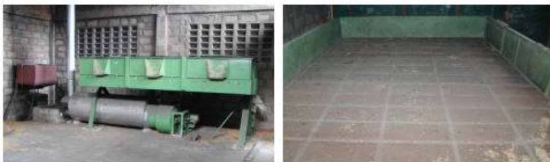
Figure 14: Kerosene fired tilted-bed dryer for easy unloading (left), drying bin with perforated false floor (right)
