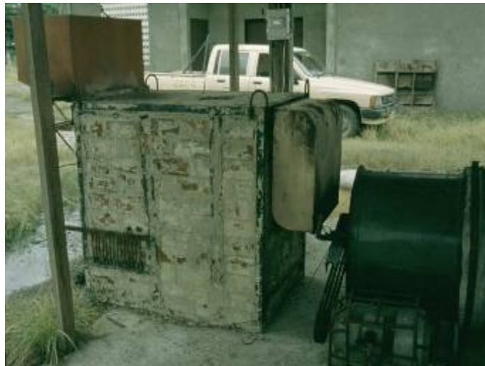
Figure 27: A simple Vietnamese inclined grate rice hull furnace for a flat bed dryer with 6-8 t capacity
