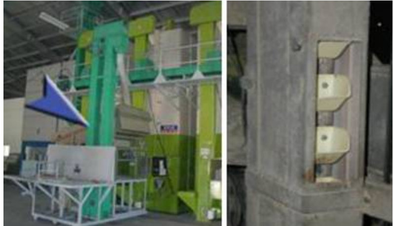
Figure 32: Bucket elevators on re-circulating batch dryers
