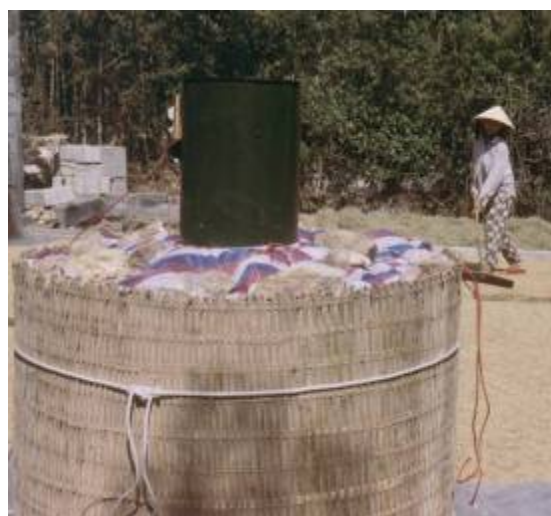
Figure 15: Vietnamese low-cost dryer with circular drying bin made from locally available materials,
