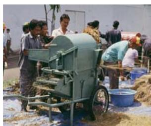
Because of high labor requirement of manual threshing stationary threshers of different types and sizes are increasingly being used.
