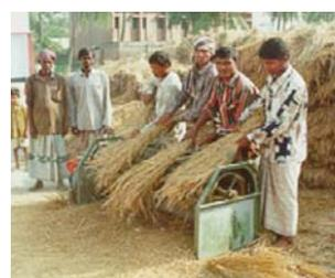
Holding the crop against a threshing drum driven by a foot crank combs the grains from the straw. Because small straw, chaff and foreign matter drops with the grains cleaning is needed.
