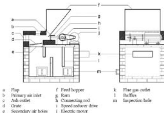
Schematic diagram of the automatic downdraft rice husk furnace.
