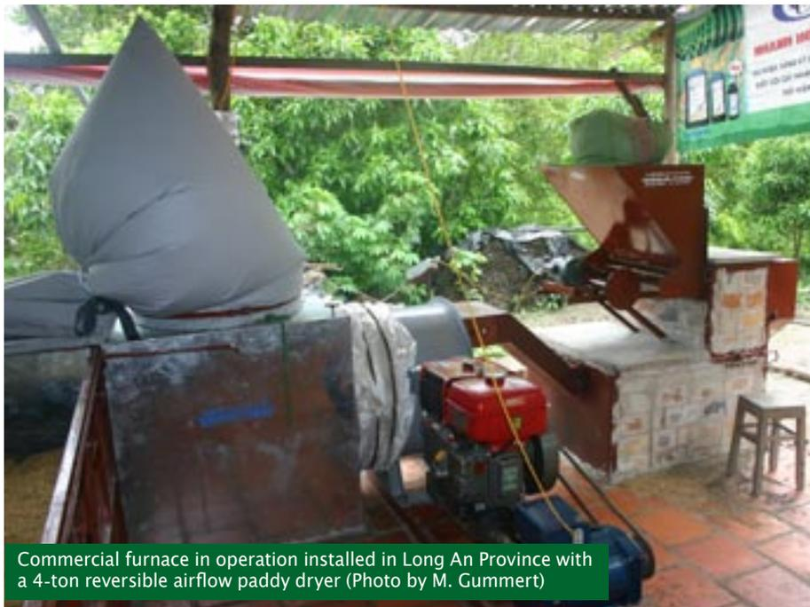
Commercial furnace in operation installed in Long An Province with a 4-ton reversible airflow paddy dryer (Photo by M. Gummert)
