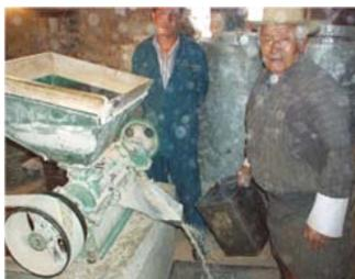
The single pass rice mill is an adaptation of the "Engleberg" coffee huller. This type of mill is still very popular in many of the poorer rice-growing countries and is widely used for custom milling of household rice. This mill is a steel friction type mill and uses very high pressure to remove the hull and polish the grain. This results in many broken kernels, low white rice recovery of 50-55% and head rice yields less than 30% of the total milled rice. The fine brokens are often mixed
