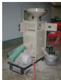
hulling and the polishing processes. Rubber rollers remove the husk and the brown rice is then polished with a steel friction whitener. These mills have a capacity of 0.5 to 1 ton per hour paddy input and are often used for custom milling in the rural areas. The milling
