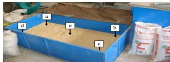
Fig. 2 SRA-500 dryer and sampling position.
