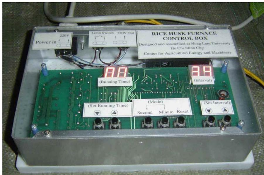
Figure 7: Microprocessor-controlled timer for the ram drive (NLU).
