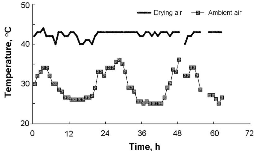
**Figure 8: Test results of the furnace at Tay Ninh in long-term operation (Phan 2005-II).**
