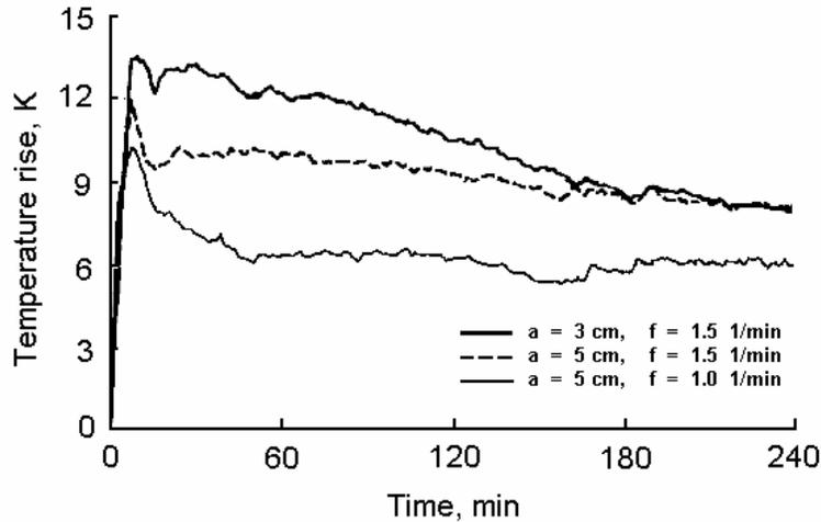
**Figure 2:** Temperature rise of the drying air in long-term operation at different piston strokes (a) and frequencies (b) (Braunbeck 1998).
