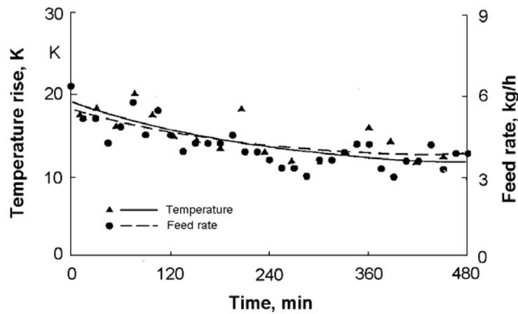
**Figure 4: Temperature and feed rate over time, Vietnamese prototype (Bojarkski 1998).**
