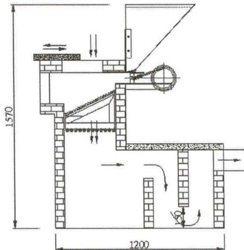
**Figure 5: Vietnamese furnace with 25-kg/h feed rate (Phan Hieu Hien 2005-I).**
