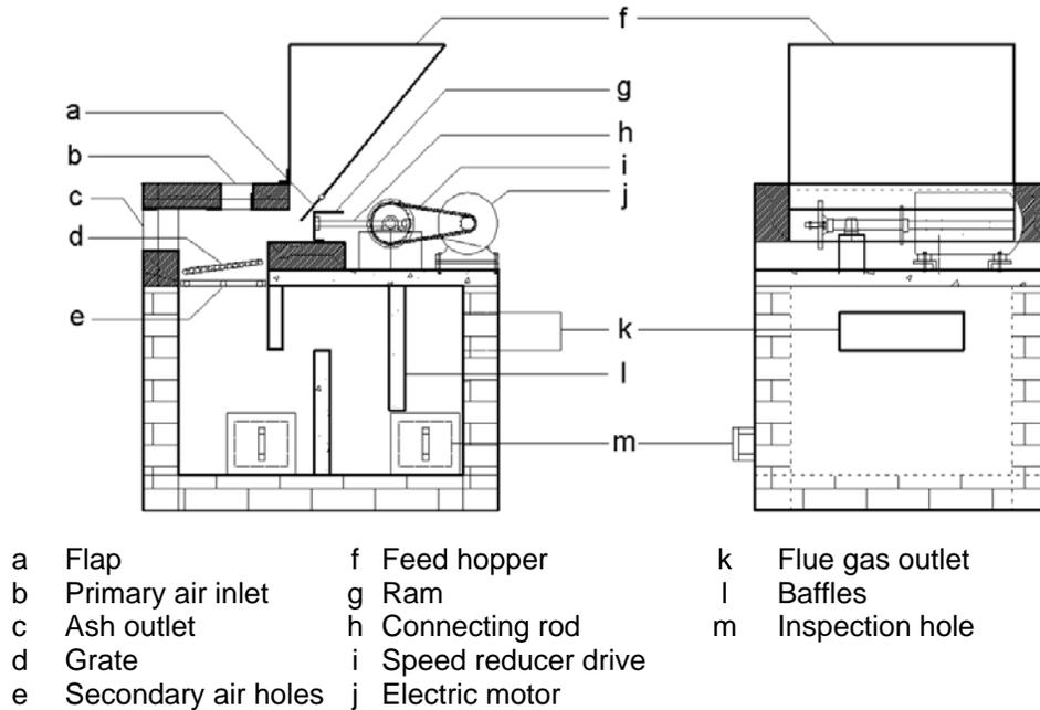
**Figure 12: The commercial prototype installed at PhilRice (modified from Chandrasekar 2005).**
