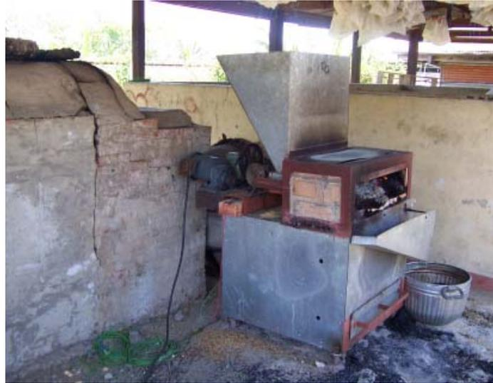
**Figure 9:** Concept prototype of a mobile rice husk furnace, test setup of a 4-t flat-bed dryer with a temporary ash collection container. On the left is the conventional manually fed inclined-grate furnace with the same capacity.
