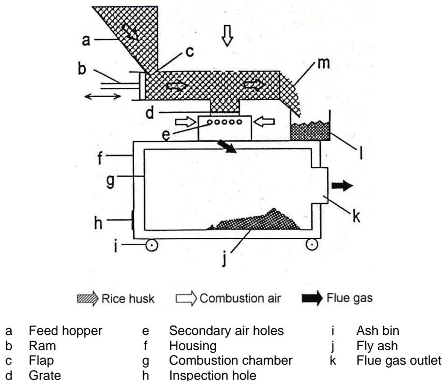
**Figure 1:** Schematic diagram of the Hohenheim furnace prototype (adapted from Braunbeck 1998).
