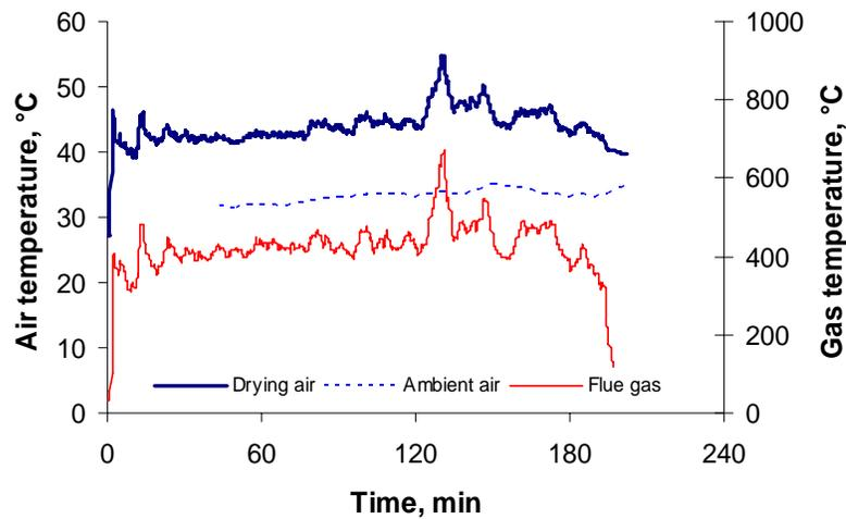
**Figure 13:** Temperature rise generated by the commercial prototype; the peak at 124 minutes was caused by overfeeding due to a breakdown of the electronic controller.
