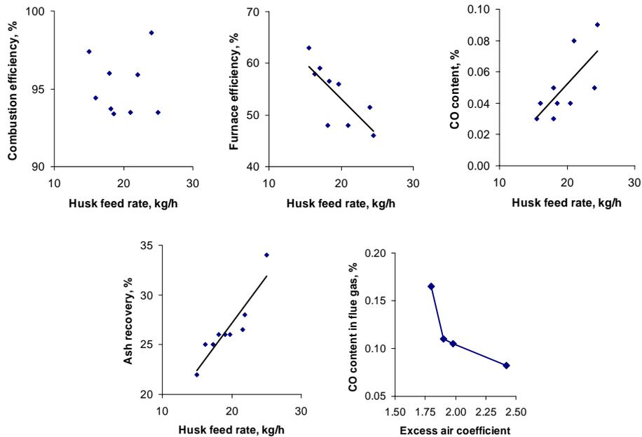
**Figure 11: Results of furnace testing: effect of feed rate on combustion efficiency, effect of feed rate on furnace efficiency, effect of feed rate on CO content, effect of secondary air, and degree of combustion.**
