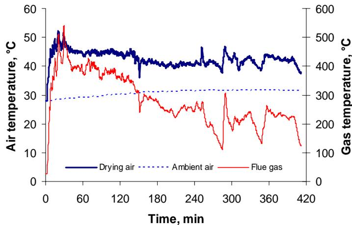
**Figure 10:** Temperature of drying air, ambient air, and flue gas over time (data from Chandrasekar 2005).
