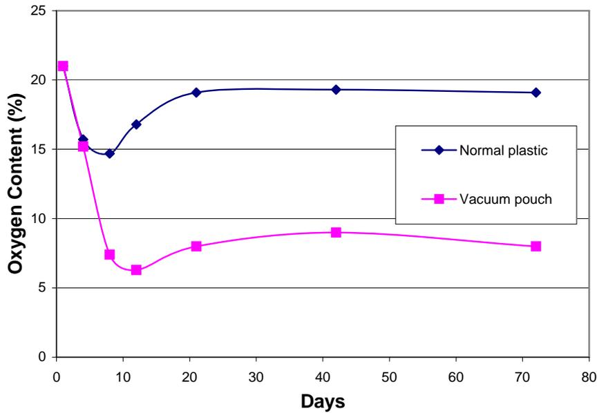
Figure 3. Change in oxygen levels in traditional plastic and medium barrier vacuum pouches
