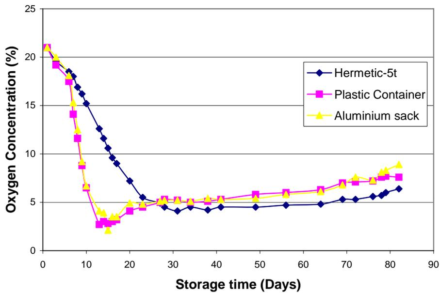
Figure 1. Reduction in Oxygen levels for the 5-ton hermetic system, 25-liter plastic container and the aluminum lined Joseph sack
