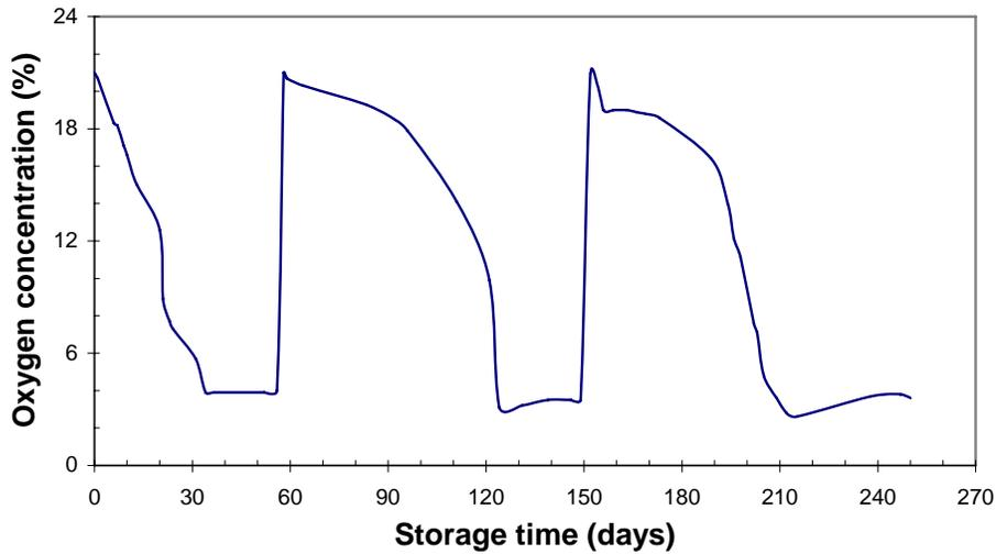
Figure 2. Reduction in Oxygen levels after opening and closing the 5-ton hermetic system.
