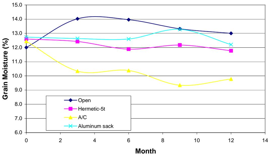
Figure4. Grain moisture content for different storage systems in the Philippines (2002-3)
